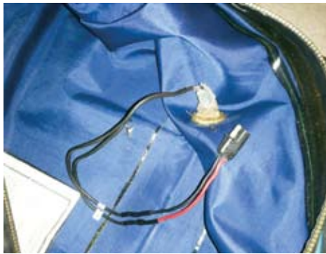
View of Marshall dry suit fitting inside dry suit. Silicone buildup placed around wires for strength, but still flexible. Connector installed which mates with vest (wires soldered and strengthened with shrink wrap). Photo by Chris Hill
