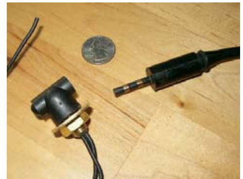
Marshall dry suit fitting on left. Marshall male wet connector on right. Photo by Bob Koch.
