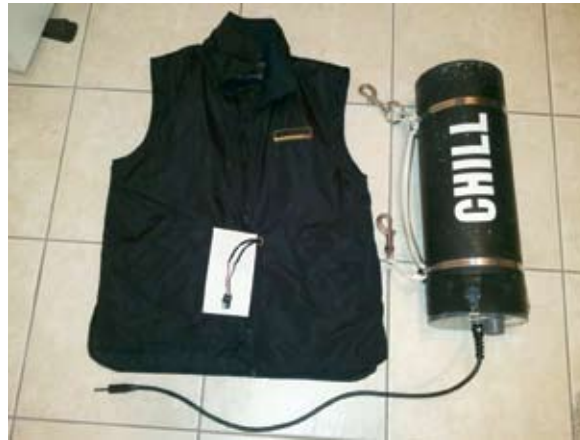
Gerbing heated vest. I've installed a grommet to route the wiring through the vest rather than hanging out the bottom. Large lead acid battery pack with Marshall cable installed. Photo by Chris Hill
