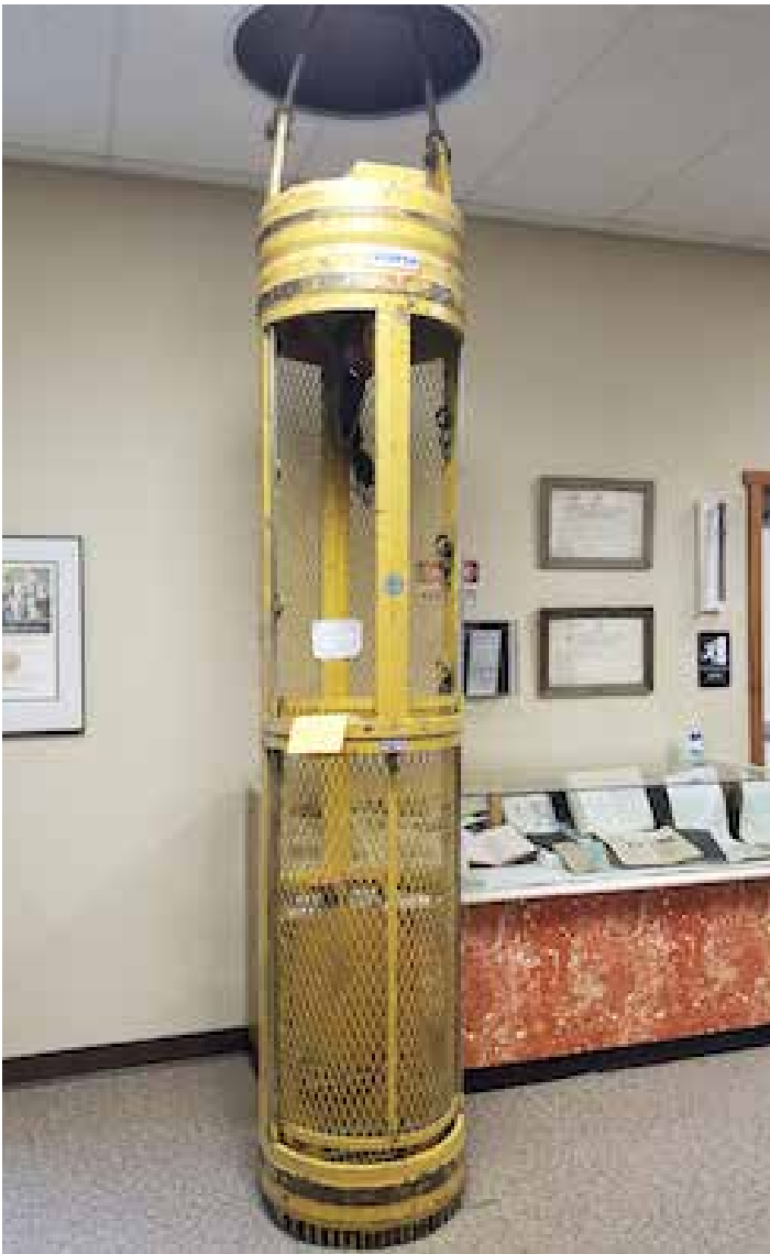
The 22-inch capsule used to rescue the Quecreek miners in July 2002. © Michael Raymond
