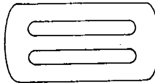
Fig. 1 Buckle. It Is Used To Hold Webbing Inside Cave Pac.
